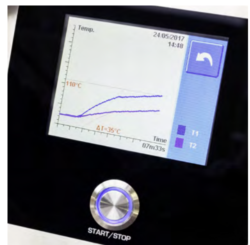
Fig. 5 A completed heating cycle with a specified Delta-T, ensuring a safely heated workpiece.
